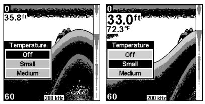
Temperature menu (left). Temperature display set to small size (right). To display Temperature:
